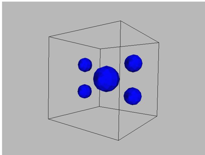
Figure 6. The Scheme of the MMC Model with five SiC Particle
