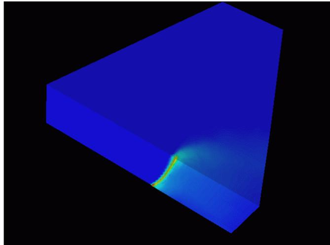
Figure 3. The Distribution of Equivalent Plastic Strain
