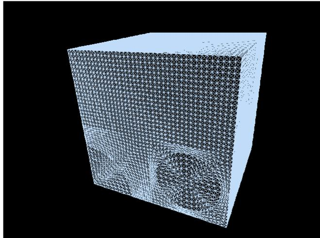
Figure 7. The Mesh Pattern of One-million DOFs FEM Model
