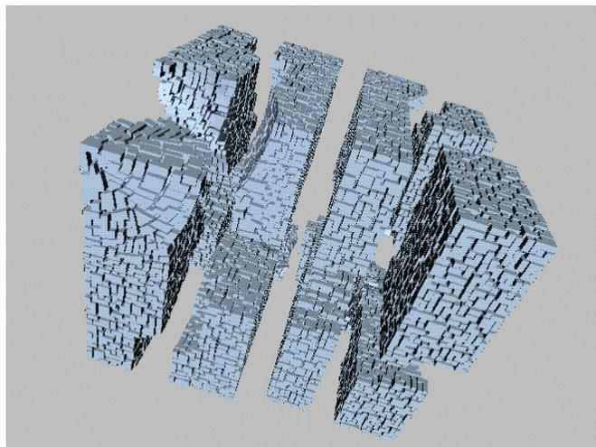
Figure 8. The Appearance of Decomposition of FEM Mesh with One-million DOFs
