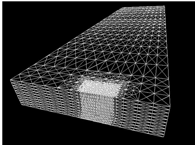
Figure 2. The Mesh Pattern of CCT Specimen
