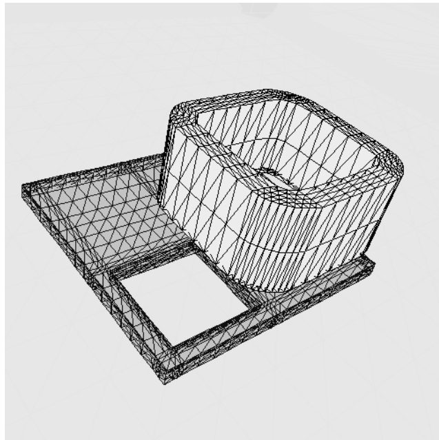
Figure 6: A finite element mesh around the coil and the conductor for the TEAM model.
