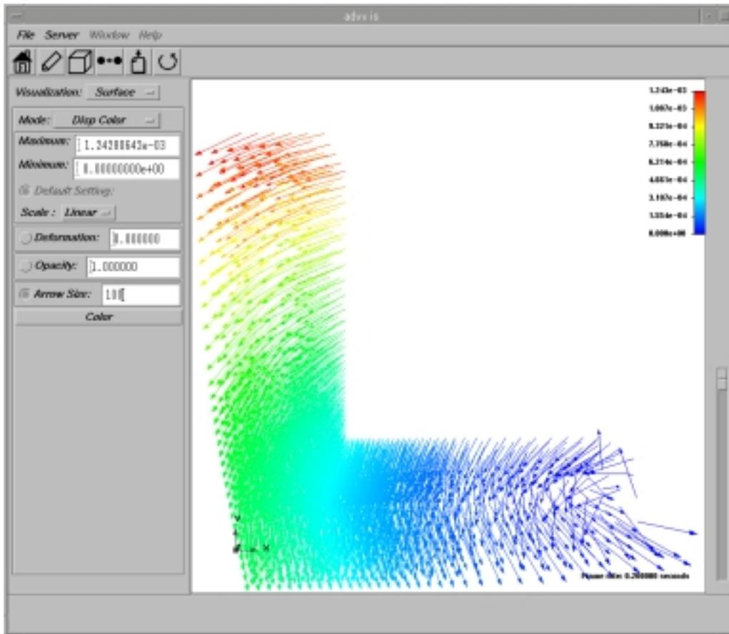
Fig. 7-15. Displacement Distribution Display (color)
