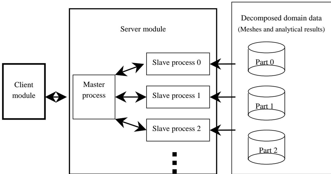
Fig. 3-1. Structure of Modules
