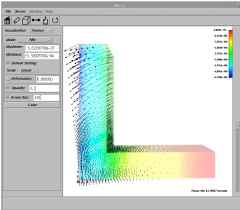
Fig. 7-17. Half-transparent Display (Opacity = 0.3)
