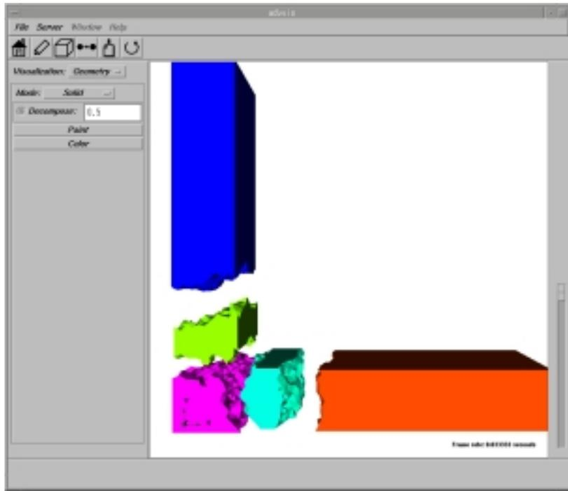
Fig. 7-7. Domain Decomposition Display (for Decompose factor = 0.5.)
