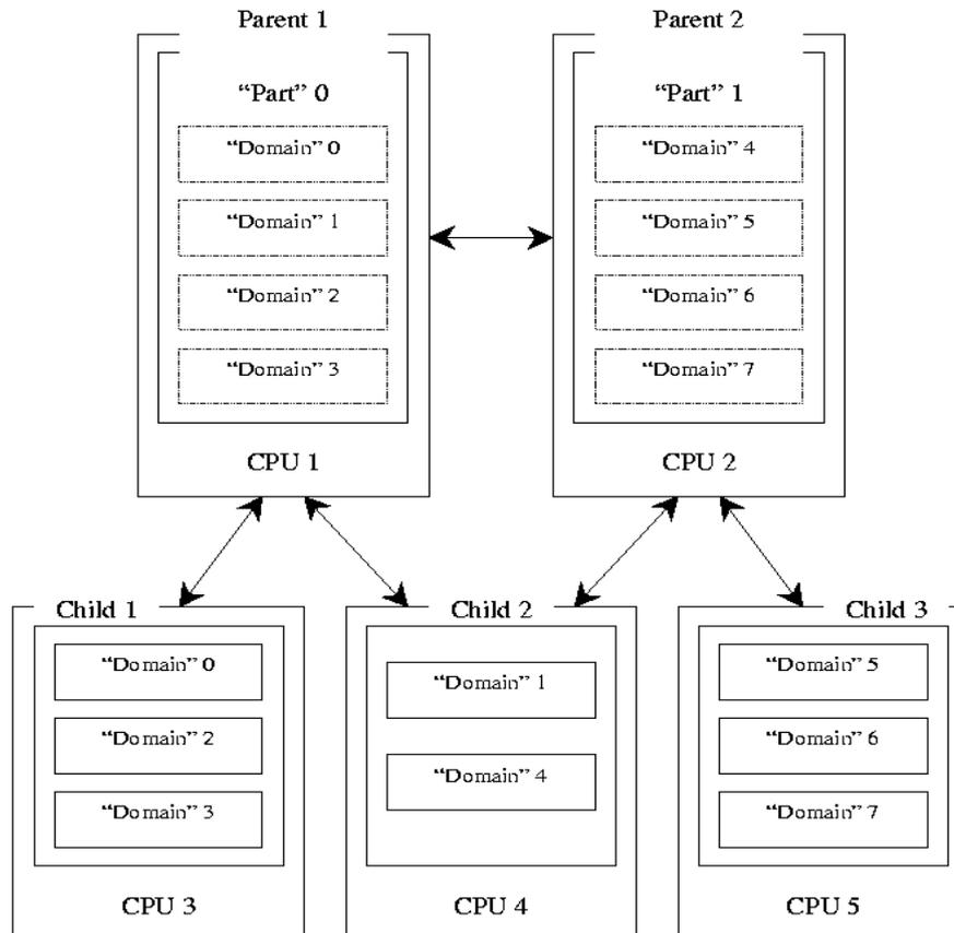
Figure 4. Adjustment of Domains to CPUs (Dynamic load distribution version)
