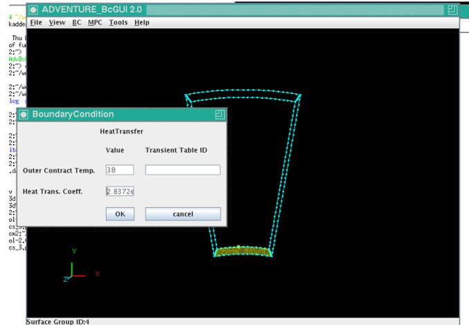
Figure 16. Example of convection boundary condition set up
