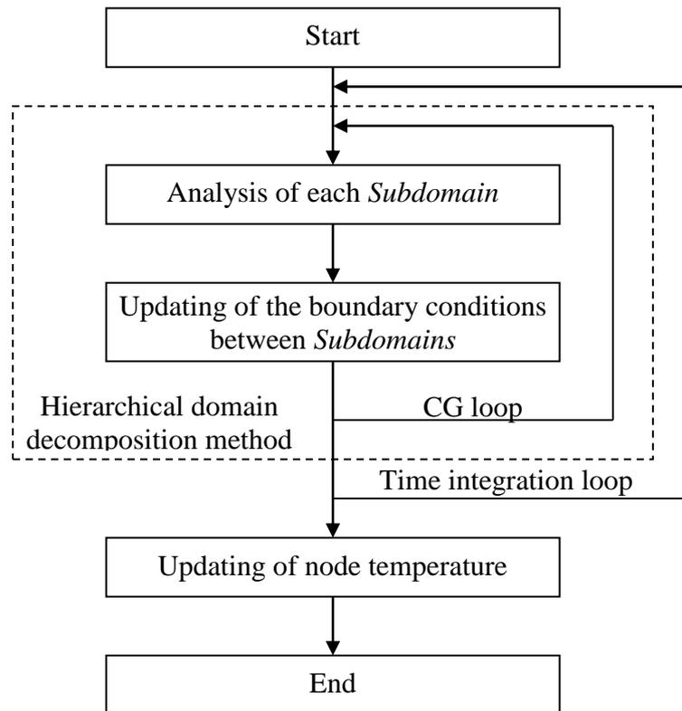
Figure 6. Algorithm of Transient Analysis
