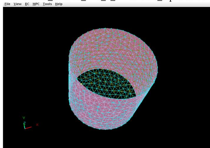
*Figure 21. Example of convection boundary condition set up at the outer surface*
