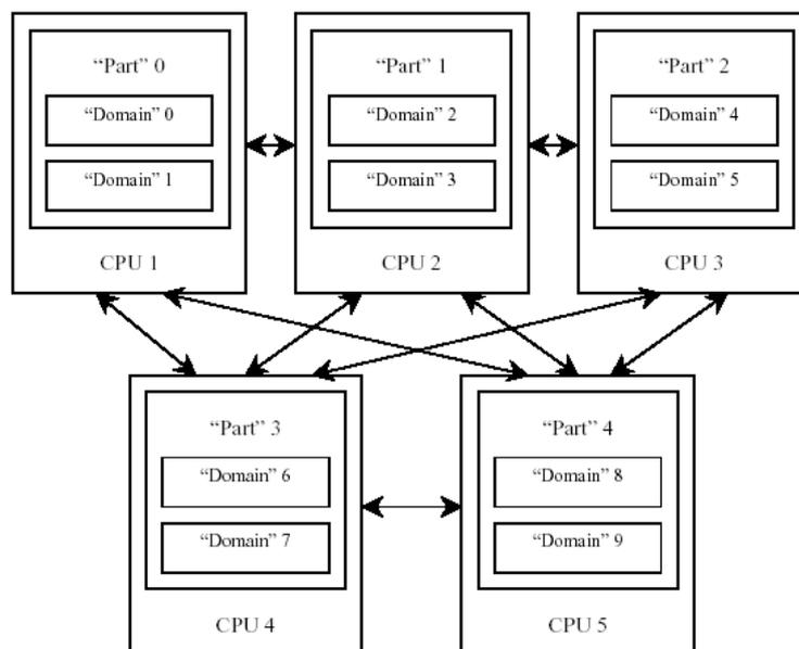
*Figure 3. Adjustment of Domains to CPUs (Static load distribution version)*
