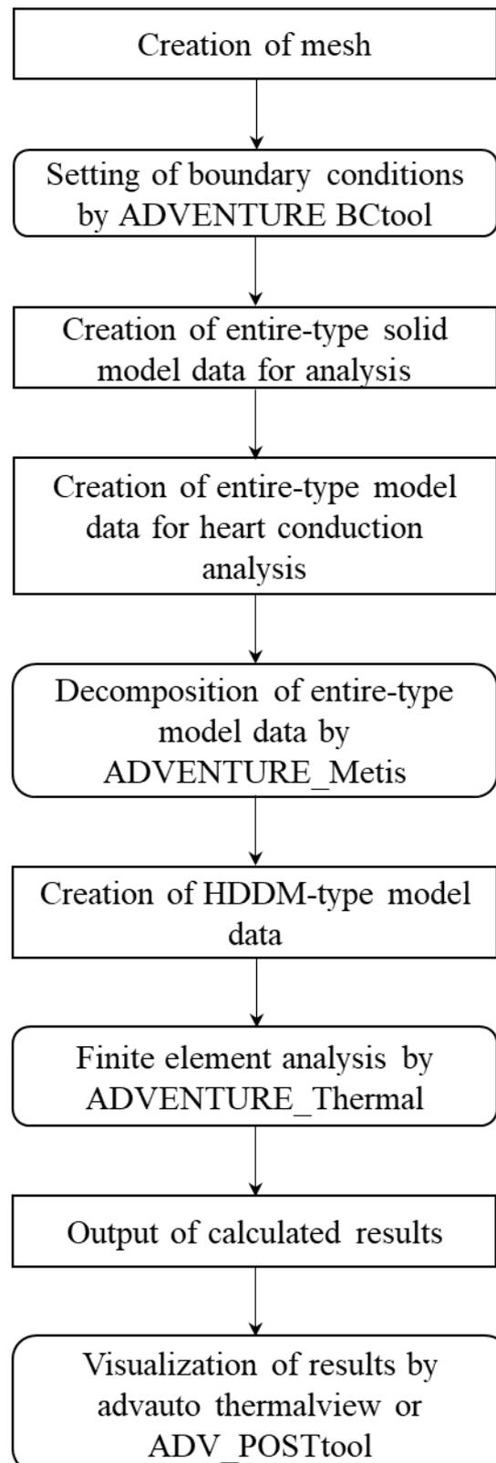
Figure 5. Algorithm of Analysis Using ADVENTURE\_Thermal Module.
