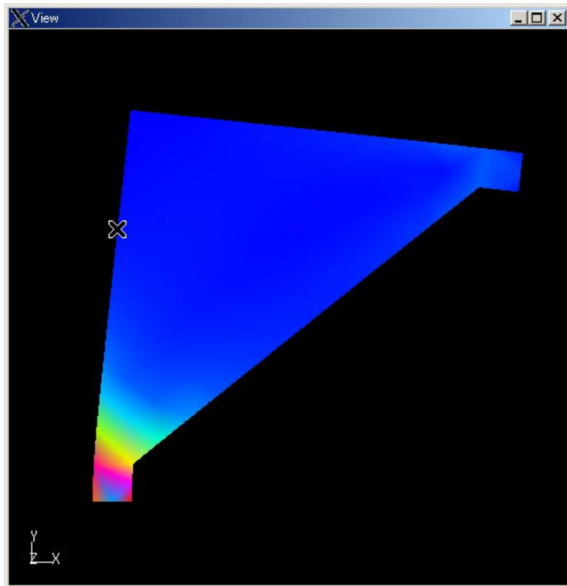
Fig. 8.2-3 Deformed geometry and equivalent stress distribution at initial parameter values
