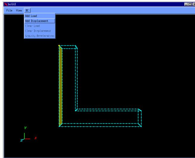
Fig. 6. Menu for Boundary Conditions Setup
