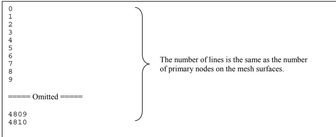
The global index file contains tabulated data where the node number of the surface patch data file (extension pch) is converted to the node number of the mesh data file (extension msh). The line number  $N$  in a global index system corresponds to the line number  $N-1$  of a local index system.
