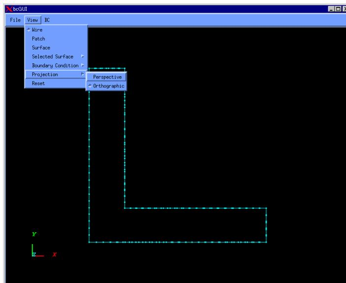
Fig. 29. Switch to Perspective Projection View
