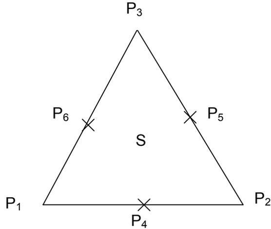
If the load distributions  $f_1 \sim f_3$  are given for the area of the triangular surface group  $S$ , the load  $L_1$  concentrated on the node  $P_1$  will be
