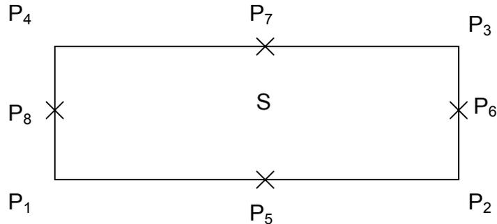
If the load distributions  $f_1 \sim f_4$  are given for the quadrangle face group area  $S$ , the load  $L_1$  concentrated on the node  $P_1$  will be
