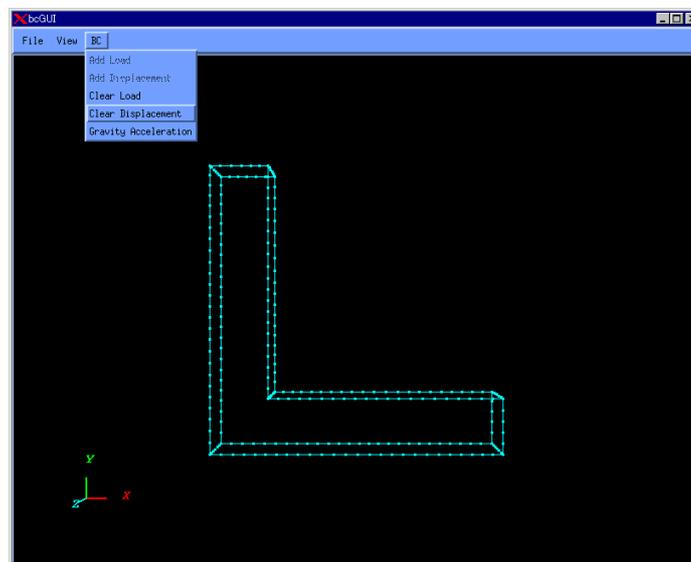
*Fig. 16. Removing of All Set Displacements*
