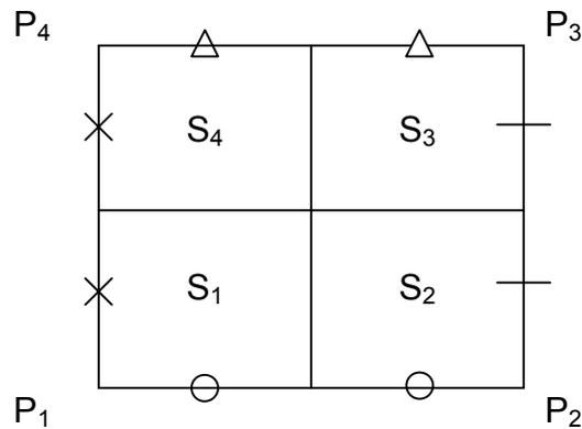
If the load distributions  $f_1 \sim f_4$  are given for the face groups areas  $S_1 \sim S_4$  respectively, the load  $L_1$  concentrated on the node  $P_1$  will be
